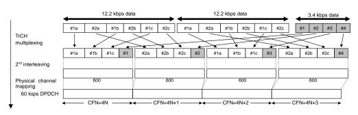
Figure 3.1.2-2 Channel coding and multiplexing for UL AMR TFCSx (2 of 2)
