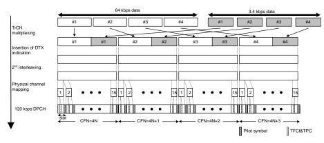
Figure 3.1.5-3 Channel coding and multiplexing for DL ISDN
