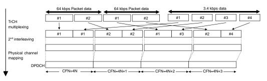
Figure 3.1.2-6 Multiplexing for UL 64 kbps packet
