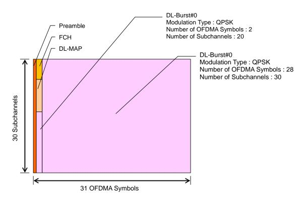
Figure 3.14.1-1 WiMAX\_DL\_10MHz\_QPSK Frame Composition
