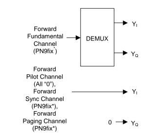
Figure 3.8.8-1 Signal generation block diagram of waveform pattern FWD\_RC3-5 9channel (1/2)
