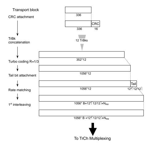
Figure 3.1.5-4 Channel coding for DL 384 kbps packet
