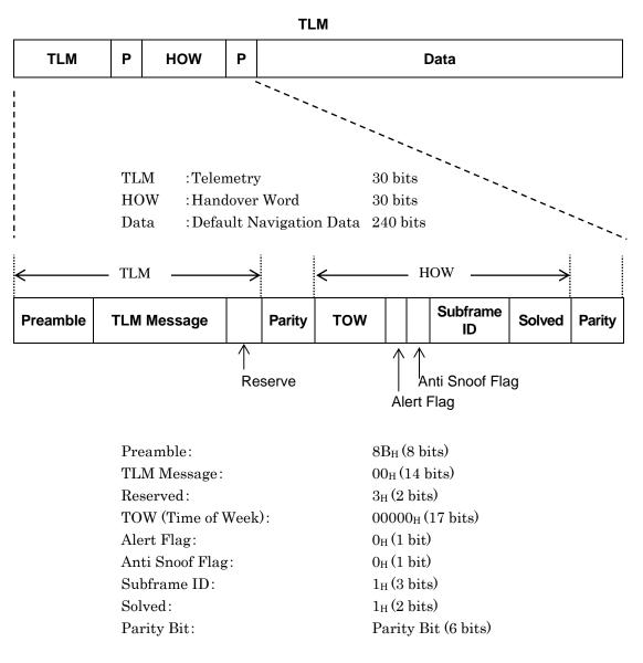
Figure 3.18.1-1 Waveform format of DefaultNavData
