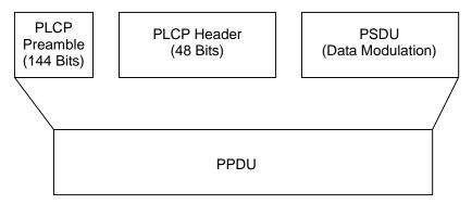
Figure 3.10.3-1 IEEE802.11b Long preamble PPDU frame format
