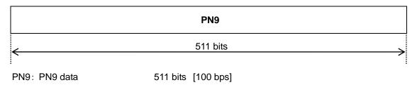
Figure 3.17.1-2 Waveform format of GLONASS\_PN9
