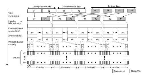
Figure 3.1.5-5 Multiplexing for DL 384 kbps
