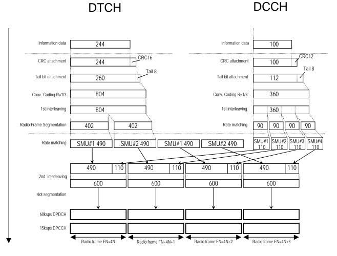
Figure 3.1.1-1 Channel coding for UL reference measurement channel (12.2 kbps)
