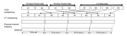
Figure 3.1.2-4 Multiplexing for UL ISDN
