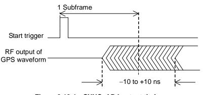
Figure 3.13-1 SYNC\_ADJ output timing
