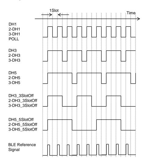
Figure 3.12-1 below shows the timing chart of waveform patterns that have a packet format.
