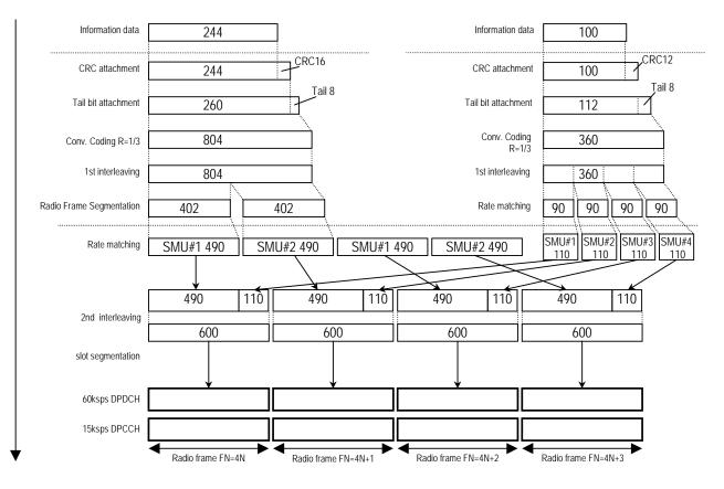
Figure 3.1.1-2 Channel coding for UL reference measurement channel (12.2 kbps)
