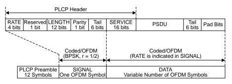
Figure 3.10.1-1 IEEE802.11a PPDU frame format
