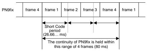
Figure 3.8.1-3 PN9fix data and short code
