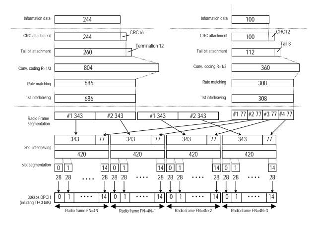
Figure 3.1.4-1 Channel coding for DL reference measurement channel (12.2 kbps)
