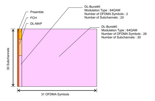
Figure 3.14.1-2 WiMAX\_DL\_10MHz\_64QAM Frame Composition
