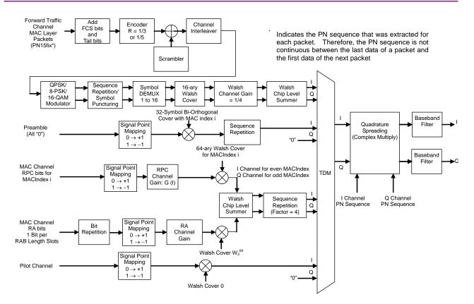
Figure 3.9.1-2 Signal generation block diagram of 1xEV-DO forward waveform pattern
